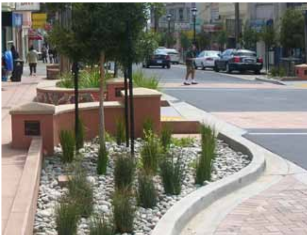
Photos, above: (1) Pedestrian crossing beacons use warning lights to alert motorists of an approaching pedestrian crossing. (2) Bulbouts create additional pedestrian space to incorporate planting, bioretention, and/or seating. Bulbouts also reduce pedestrian crossing distance. (3) Gateway entrance to Youngstown State University
